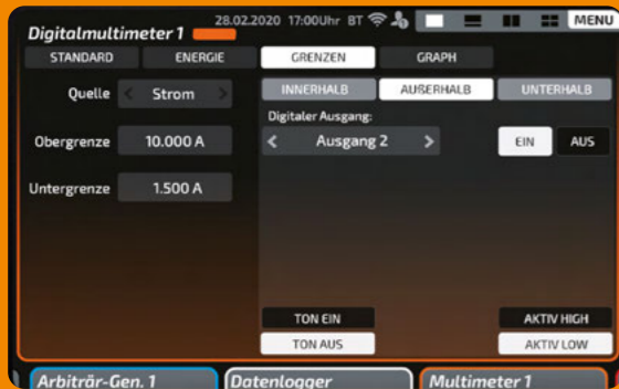
Limiter: Each measurand can be monitored by definable limits using tones and digital outputs. The digital outputs can be used directly for example to indicate different states by means of the erfi RGB indication light.
