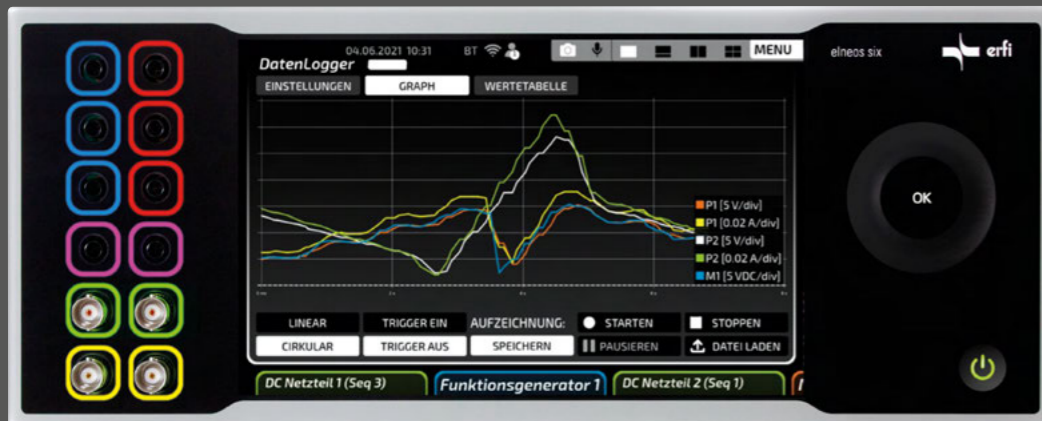
Measured value display: The data logger allows the simultaneous and synchronised graphic display of 5 different measured variables or devices, including X-Y zoom and scroll functions. Individual curves can also be hidden.
