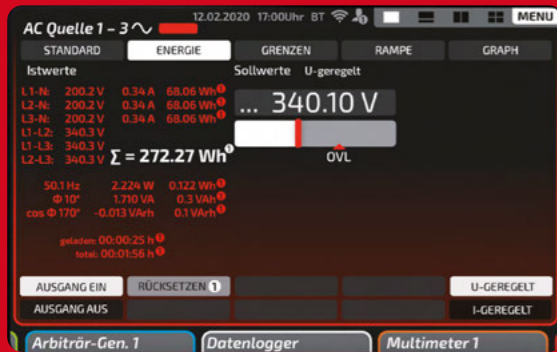
3-phase AC sources with power and energy meter: For 3-phase AC sources, a 3-phase power and energy meter is included in the scope of delivery. The actual voltages between all phases and N are displayed simultaneously.
