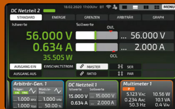
Efficient use of all equipment groups: Even if the power meter is in the small secondary range, it is possible to switch between power measurement and digital multimeter functions.
