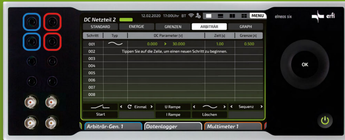
Curve parameters: Input of the different curve parameters in tabular form. AC and DC parameters are to be entered for this purpose.
