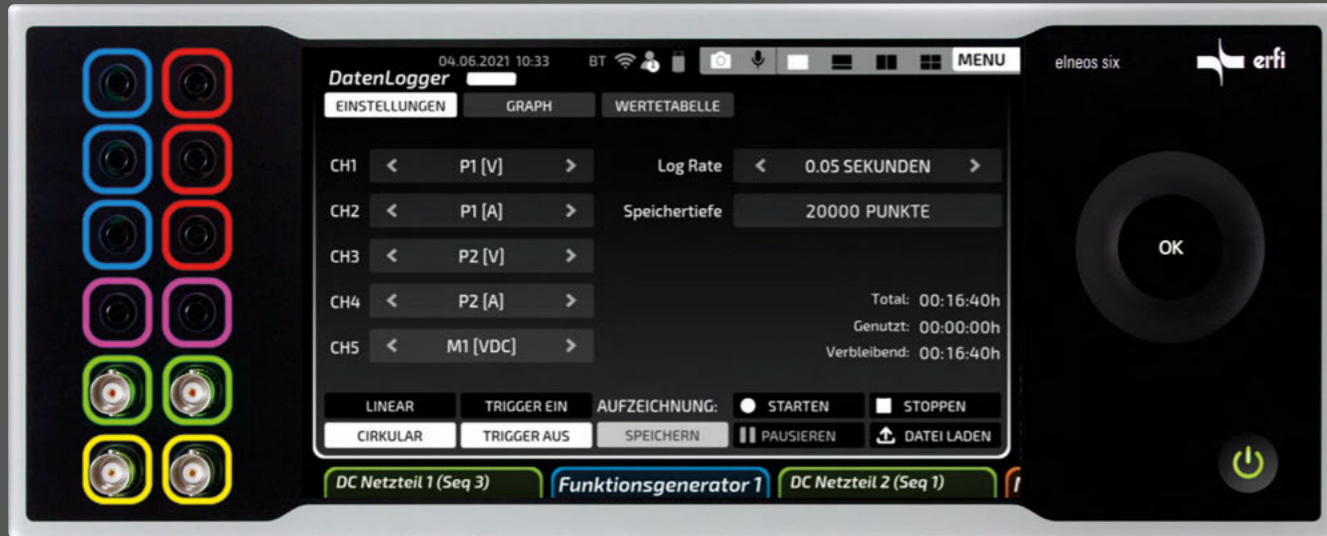
Measured value display, measuring devices (DMM, P-meter) and power supplies (AC, DC): Via the data logger, 5 different measured variables can be selected and the measuring rate and storage depth (up to 500,000 measuring points) can also be defined.
