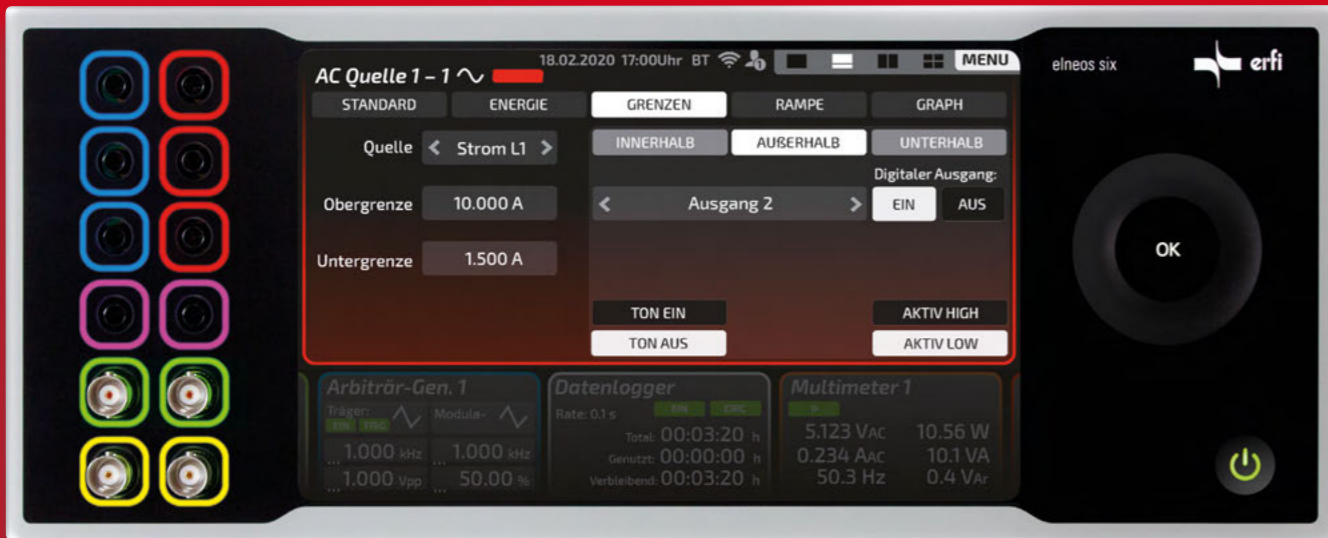
Limitier: The limiter, guarantees the monitoring of current and voltage as well as the external control of other device groups and the indication light (integrated PLC function).
