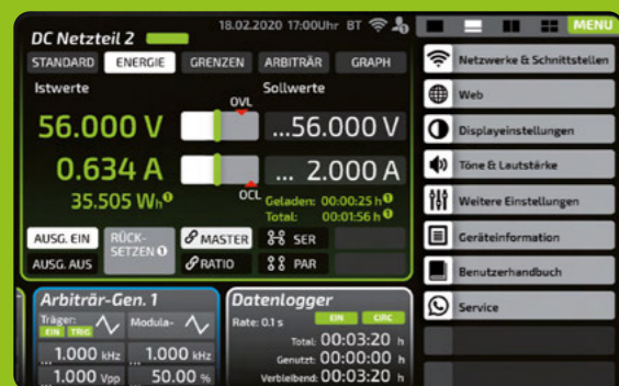
Menu bar and dynamic screen scaling: When the menu bar is displayed, the screen dynamically collapses and remains completely legible and operable during the display. Disturbing cross-fades of menus are thus completely avoided.
