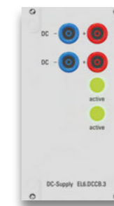
Insert plate as aluminium front for double DC sources and DC power arbitrary generators 3 U / 14 HP For direct connection to any two DC sources. Control by control centre via rear e-bus. Note: Power output stages of the power supply units either in the 19-inch unit cockpit, in the 19-inch table-top unit or in the TechCube (under-table installation). Output: 4 SLS 1 (2 per DC source) Display: RGB-LED for Output active Order no. EL6.DCCB.3
