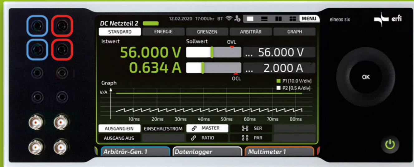
2/3 screen mode: Control unit in the main screen, with power display and horizontal sliders for coarse adjustment.
