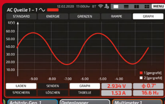
Data logger and graphic display of measured values: Visualisations and real-time recordings of freely programmable ramp functions for tracking voltage and current curves. The current values are always faded in. Alternatively, the data can be displayed in tabular form.
