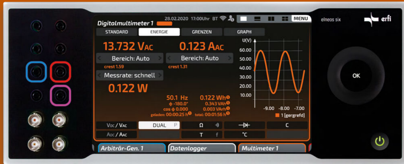
Power and energy measurement: The power and energy meter in full-screen mode with Display of all relevant energy values as well as the active energy and the crest factors for U and I incl. zoom function.
