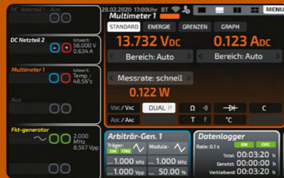
Connection panel with actual value display: The new connection panel shows all measured values at the outputs and inputs. The screen with the unit displays scales automatically. The connection panel thus represents a separate information screen that can remain permanently displayed.
