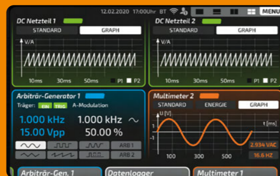
Quattro screen: The unit remains operable in each of the split screens. The graphical display of measured values can also be used and operated in parallel with other devices such as DC power supplies or AC sources in the smallest screen (Quattro screen).
