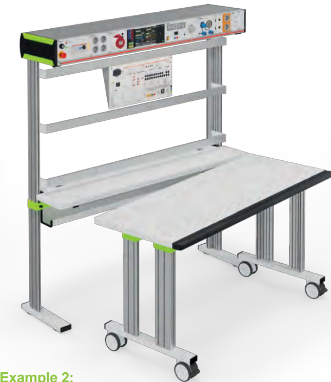
Example 2: Laboratory bench: ELC1.1.1641.C 1600 x 400 x 780 mm. Table type 1.1. ergo-line worktop (laser edge). Mobile extension table: ELC1.1.1663A.T 1600 x 600 x 780 mm. Worktop alu-line (laser edge). Structure: Extended L-profiles. 19-inch cockpit, equipped with the basic and elneos six device series. 2-row experiment frame between the base profiles. Cable aperture sockets embedded in the table top, open cable tray underneath the table.
