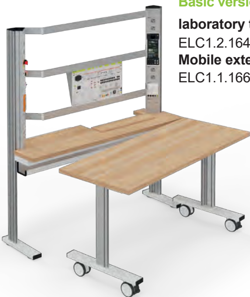
Example 3: Laboratory bench: ELC1.2.1648.C 1600 x 400 x 780 mm. Table type 1.2 with 180° cable flap. Optional split cable flap. Multiplex worktop. Mobile extension table: ELC1.1.1668A.T 1600 x 600 x 780 mm. Worktop multiplex. Connectors each in graphite black, RAL 9011. Structure: Extended L-profiles with Expand 2 profiles on the left and right, fitted with the acto and elneos six compact device series. 2-row experiment frame between the base profiles.
