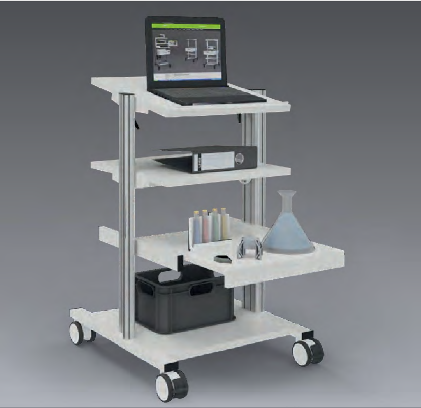
Fig. 1 left: Orgamobil (W x D x H): 721 x 758 mm x 1100 mm Usable area (W x D): 600 x 600 mm With inclinable shelf, straight shelf and pull-out shelf.
