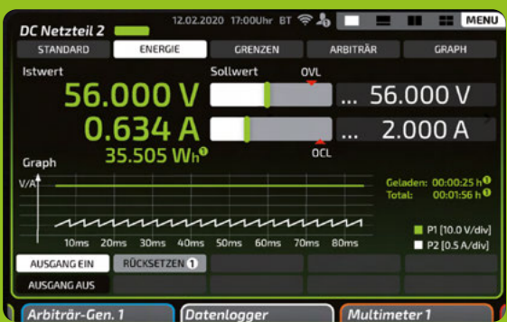
Energy meter: The new control power supplies record the power graphically and numerically at any time.
