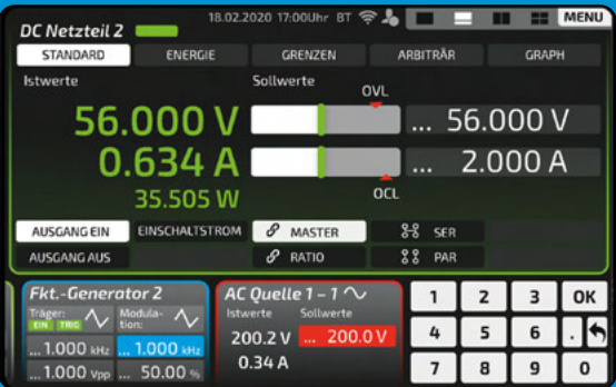
Comfortable access: Even in the smallest screen, the 8-inch display allows values to be entered using the keyboard, wheel or rotary encoder.
