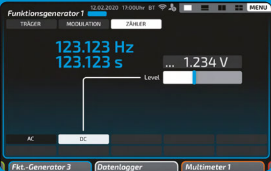
Built-in counter: Allows the acquisition of AC and DC signals as well as the setting of the trigger level in the DC range in the standard up to 150 MHz. Optional increase of the measuring range to 1.5 GHz.
