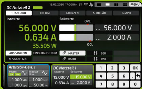
2/3 screen mode: Control setting unit in small window with numeric keypad. Even in the small window, the units can be operated and setpoints can be entered.
