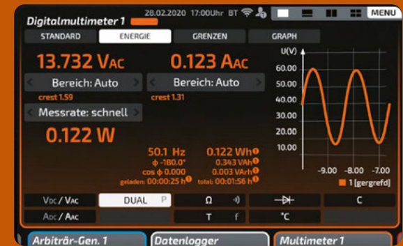
More scalable graphic measured value display: In the upper half, the power meter displays all measurement data. At the same time, in full-screen mode, other devices can be displayed in the smart scroll bar.
