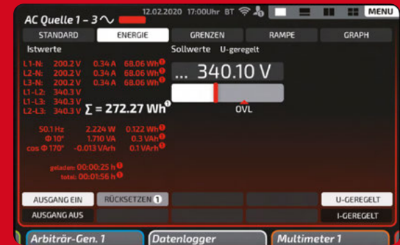
3-phase AC sources with power and energy meter: For 3-phase AC sources, a 3-phase power and energy meter is included in the scope of delivery. The actual voltages between all phases and N are displayed simultaneously.
