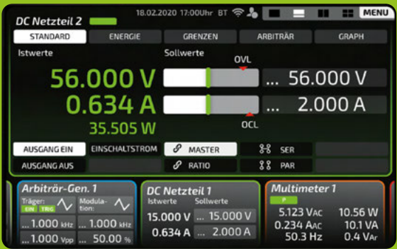
2/3 screen mode: After entering the values, the device bar can be easily moved by swiping gestures on the display or by 3D gestures (Smart scroll). The devices glide elegantly horizontally across the screen.
