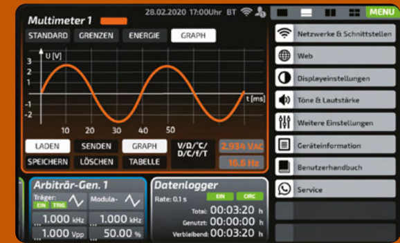
Dynamic screen content: When menus are displayed, the screens scale automatically without overlaying the unit displays. In this way, you always remain connected to all devices and can, for example, follow measured value progressions in parallel during parameter settings.
