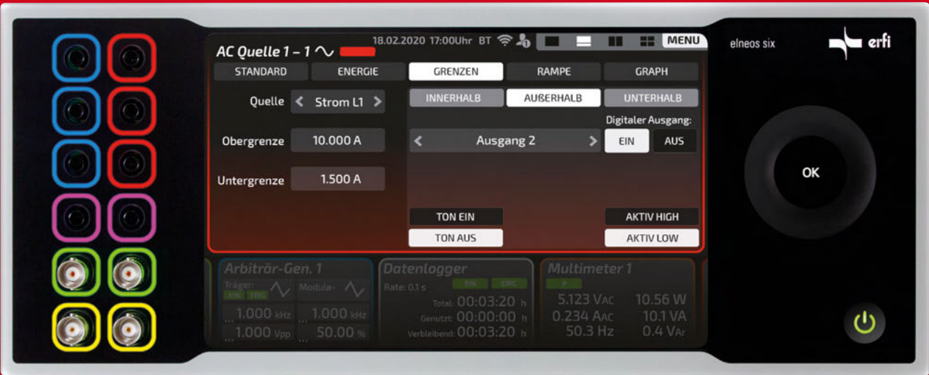
Limiter: The limiter, guarantees the monitoring of current and voltage as well as the external control of other device groups and the indication light (integrated PLC function).
