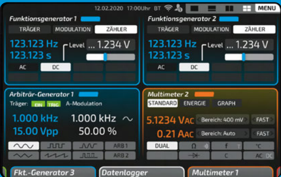
Splitscreen: In the Quattro screen, too, input is implemented by means of a slider in the display. Compared to conventional 7-inch displays, the 8-inch display shows off its full size here and enables this convenience in every device.
