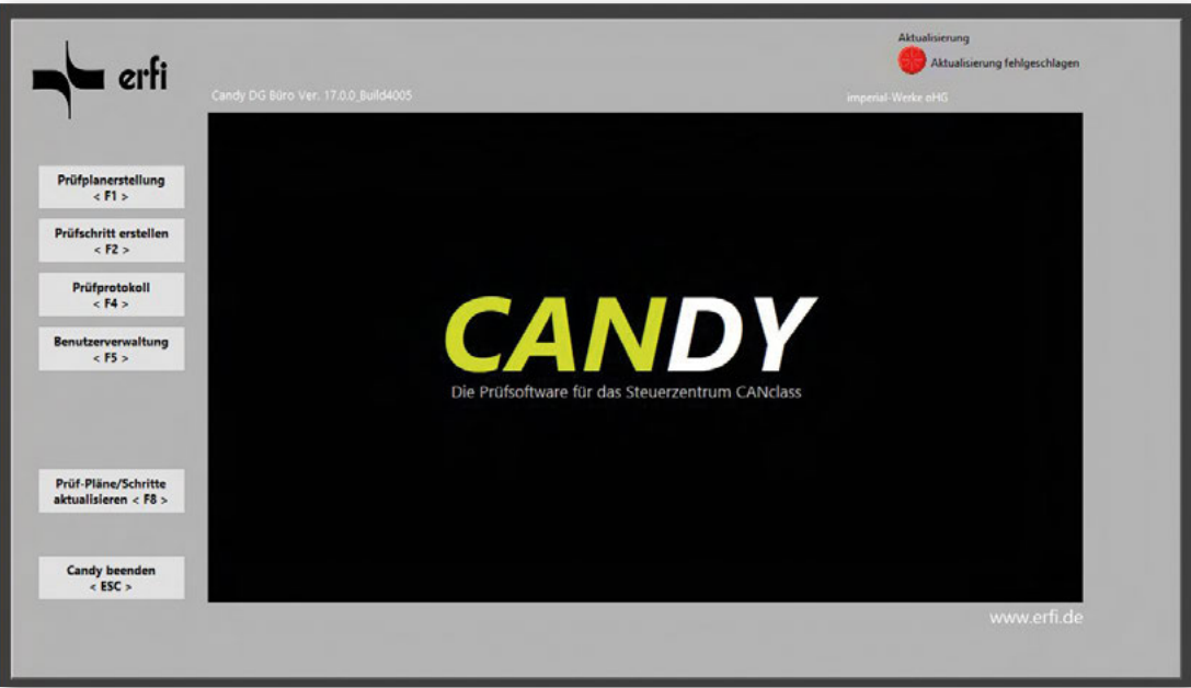
Start screen with the four main areas test planning, test procedure, test protocol and user administration.
