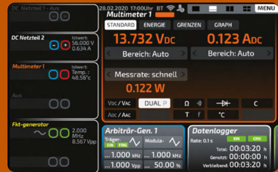
Connection panel with actual value display: The new connection panel shows all measured values at the outputs and inputs. The screen with the unit displays scales automatically. The connection panel thus represents a separate information screen that can remain permanently displayed.
