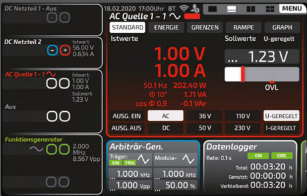
Connection panel with live measured value display: the rest of the screen is dynamically scaled when the connection panel is displayed and can always be operated in parallel.
