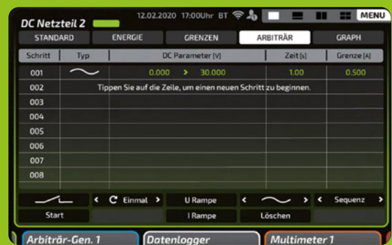
Ramp generator: Owing the 8-inch display, any sequences can be entered directly without any programming. This is a decisive advantage for daily work. Alternatively, the sequences can be transferred and started via the interface.
