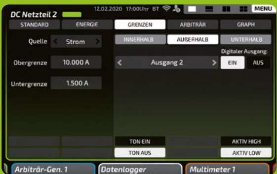
Limiter: The limiter allows the free monitoring of voltage and current ranges in conjunction with limits. Each state can be coupled with an acoustic signal and a freely selectable digital output.
