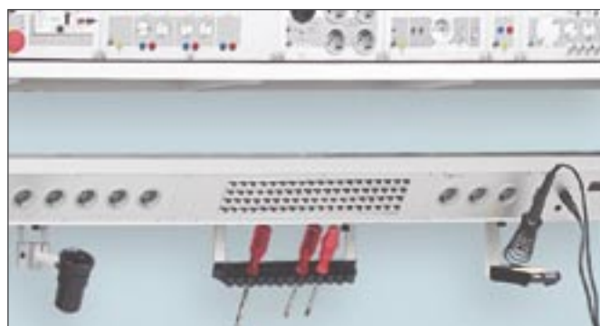
On the back of an adaptable aluminium profile further functions can be attached to the system channel such as accumulator, tool storage, perforated sheet metal plates, rotary table for small articles, device platform etc. Due to the shelf for the soldering iron, the same floats above the table top. The soldering station is installed in the system channel. This creates space and order on the working place.
