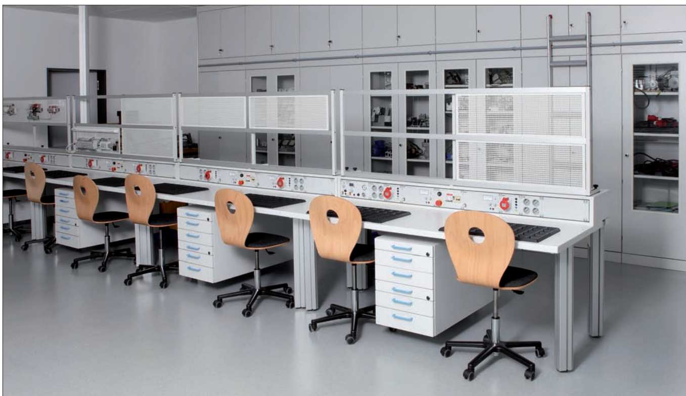
Perforated plate system for experimenting, integrated in the working place. The wall units are uncluttered and transparent due to their glass fronts.
