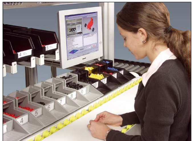
Software controlled assembly working places AWM (Assembly Workflow Management) , the Software for flexible assembly works and paperless manufacture
