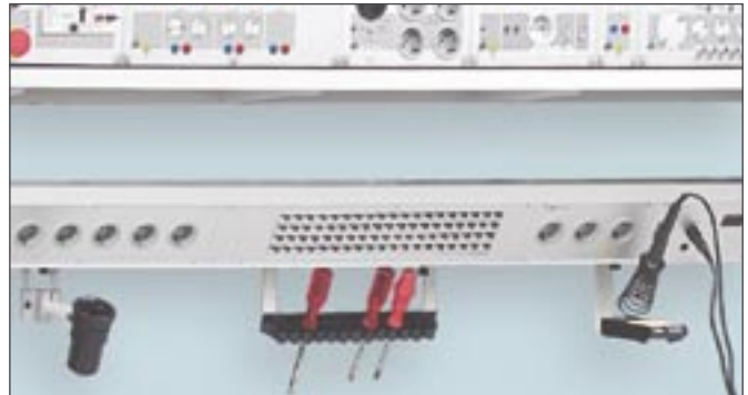
On the back of an adaptable aluminium profile further functions can be attached to the system channel such as accumulator, tool storage, perforated sheet metal plates, rotary table for small articles, device platform etc. Due to the shelf for the soldering iron, the same floats above the table top. The soldering station is installed in the system channel. This creates space and order on the working place.
