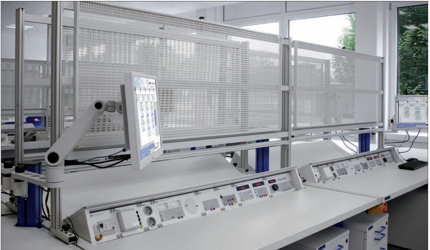
19" highlab device system with 3 HE/19" swivel attachment, movable experimenting frame with perforated plate.
