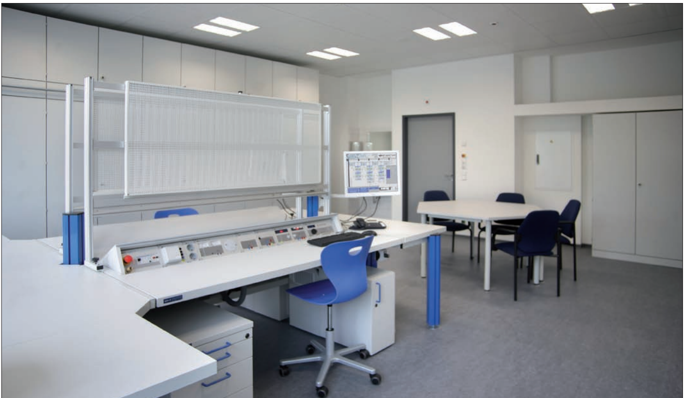
Laboratory table equipped with power pack, variable isolating transformer, function generator and many more. In the background: wall unit system and conference room with trapezoidal tables
