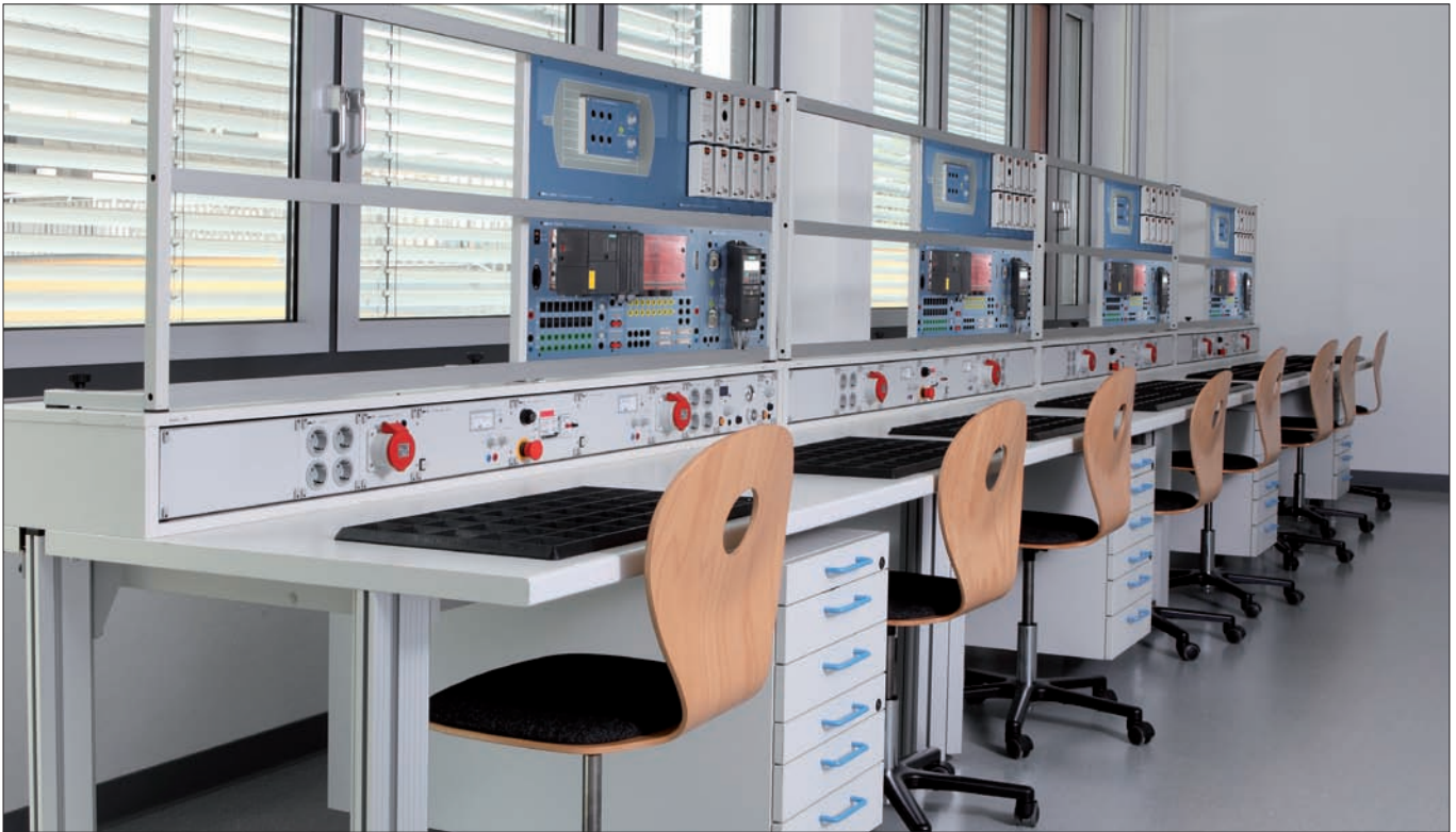
Laboratory system equipment varantec with 19" device system basic and erfi didactic teaching materials (VDE tests, motor defect simulator, PLC S7 board and frequency inverter board for the automation technology).
