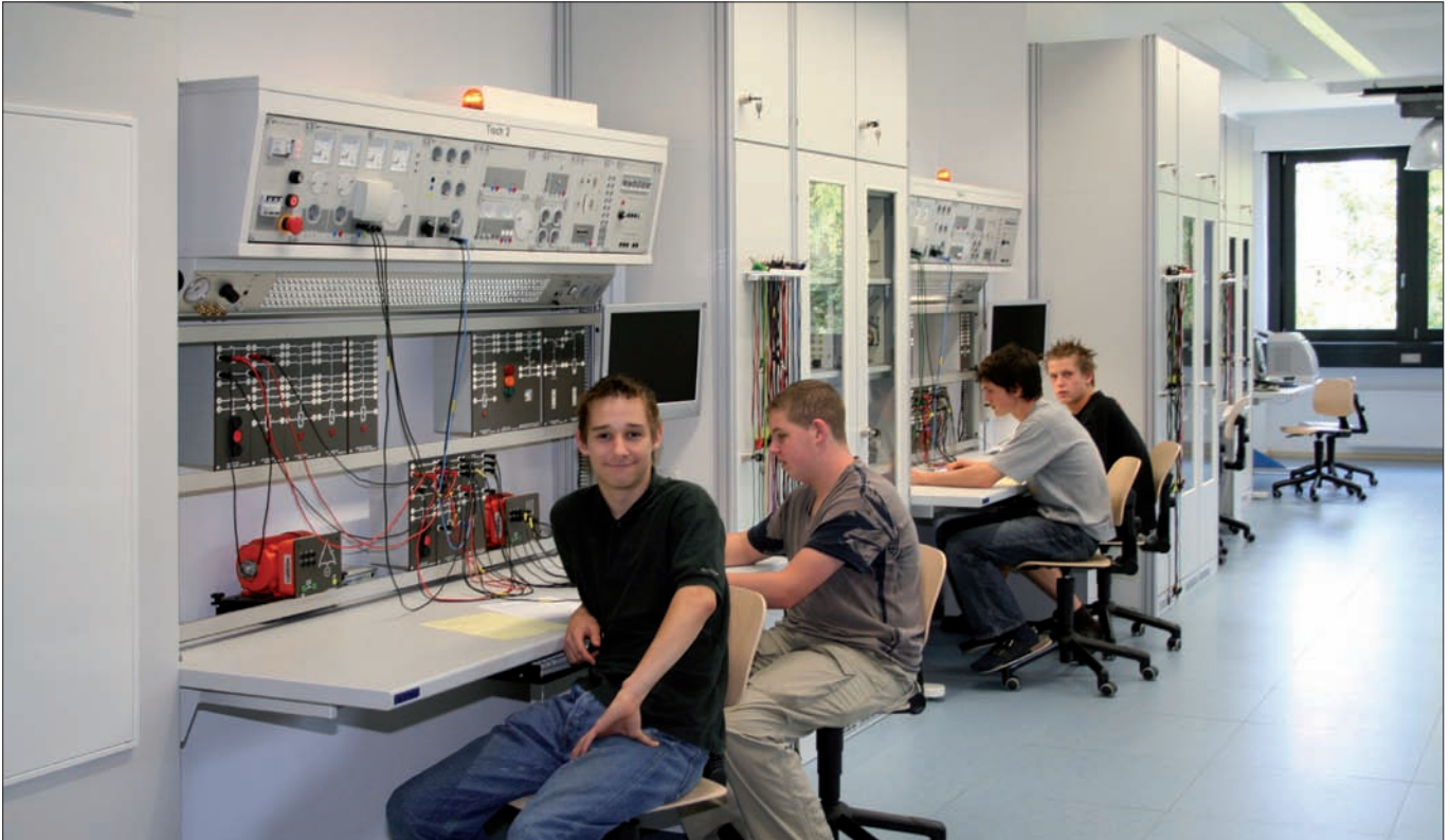
Equipment for training in the vocational training school 5 in Linz: Aluminium furniture system varantec C with integrated 19" device system highlab and aluminium cabinet system varantec select.
