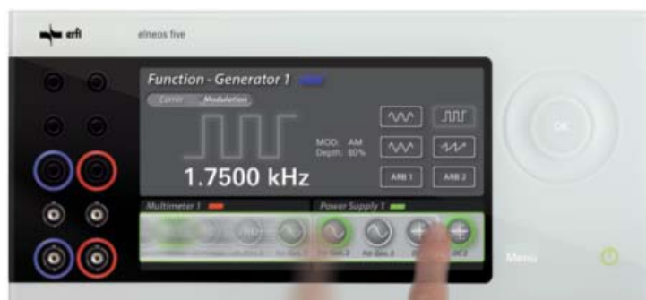
Device selection by icon device bar by 1-finger gesture.
