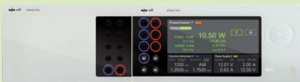
Control center + 2 arbitrary waveform generators incl. regulating power supply unit 0-30V/5A + functional generator + power and energy meter incl. digital multimeter
