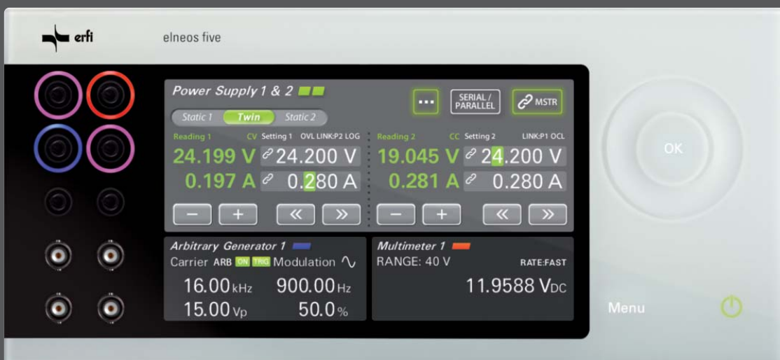
Twin operating mode in connection with the comfort equipment for ease of operation (Ref. No. EL5.C): Both options can ideally be combined and allow a high ease of use with a double power control unit.
