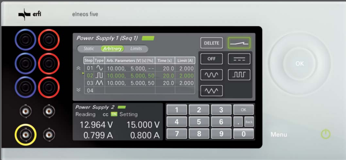
Input of the different curve parameters in tabular form. For this the AC and DC parameters must be input.
