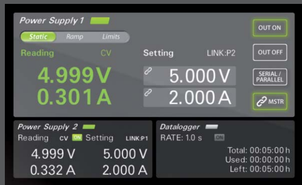
Optional added equipment (Ref. No. EL5.C): The master/slave function allows to couple two control power units. A slave control unit follows the master control unit with current and voltage.
